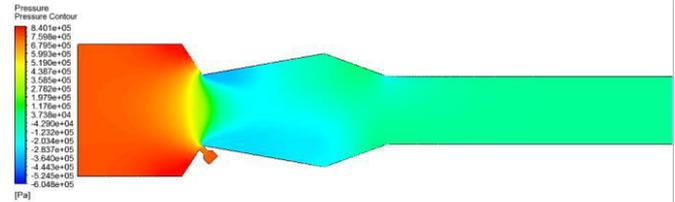
**Fig 3.1.5: pressure contour of DTN of single 135° ejector**
