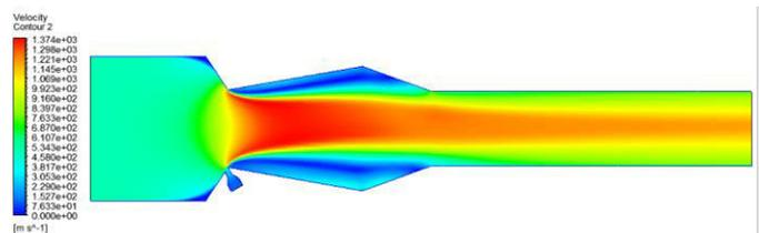
Fig 3.2.3: velocity contour of DTN of single 120° ejector
