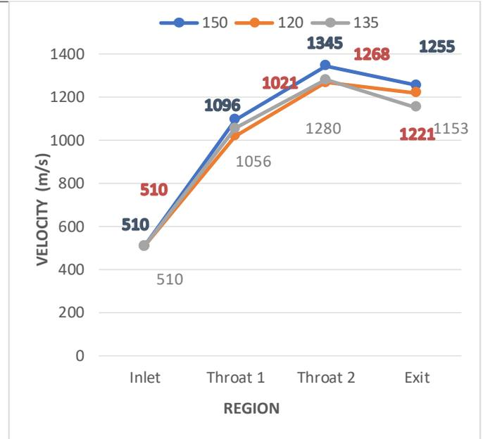
**Fig 3.2.6: velocity contour comparison of DTN with single ejector.**
