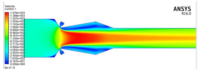
Fig 3.2.2: velocity contour of DTN of dual 150° ejector
