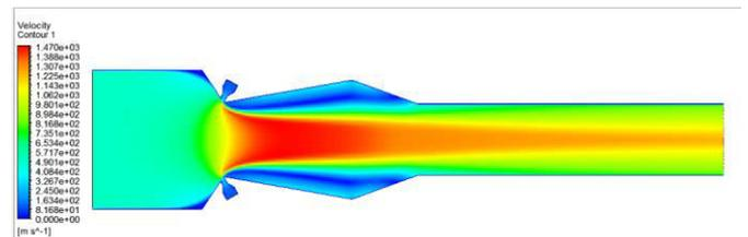
Fig 3.2.3: velocity contour of DTN of dual 120° ejector
