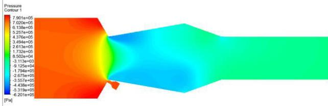
**Fig 3.1.1: pressure contour of DTN of single 150° ejector**
