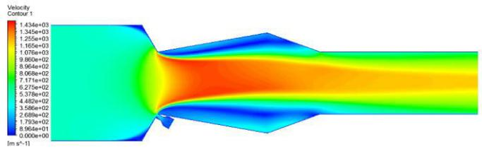
Fig 3.2.1: velocity contour of DTN of single 150° ejector
