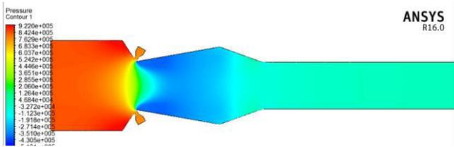
**Fig 3.1.2 : pressure contour of DTN of dual 150° ejector**
