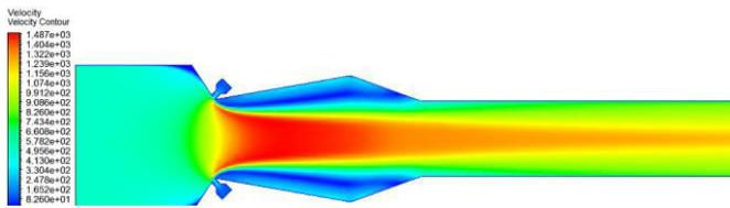
**Fig 3.2.5: velocity contour of DTN of dual 135° ejector**
