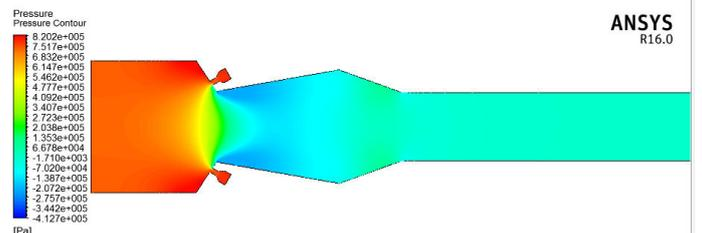
**Fig 3.1.7: pressure contour of DTN of back offset of dual 150° ejector**
