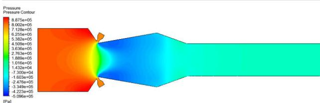
**Fig 3.1.4 : pressure contour of DTN of dual 120° ejector**
