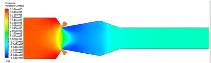
**Fig 3.1.6 : pressure contour of DTN of dual 135° ejector**
