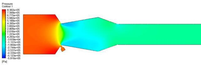
**Fig 3.1.3: pressure contour of DTN of 120° single ejector**
