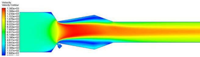
**Fig 3.2.4: velocity contour of DTN of single 135° ejector**
