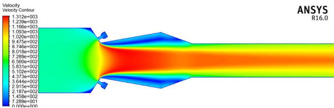
**Fig 3.2.5: velocity contour of DTN of back offset of dual 150° ejector**
